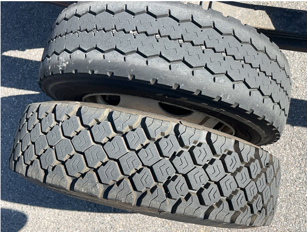
Right Inner Drive Tire Condition / Right Outer Drive Tire Condition / 08-11-2023
