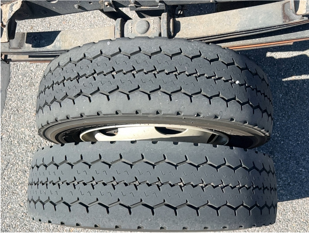
Left Inner Drive Tire Condition / Left Outer Drive Tire Condition / 08-11-2023
